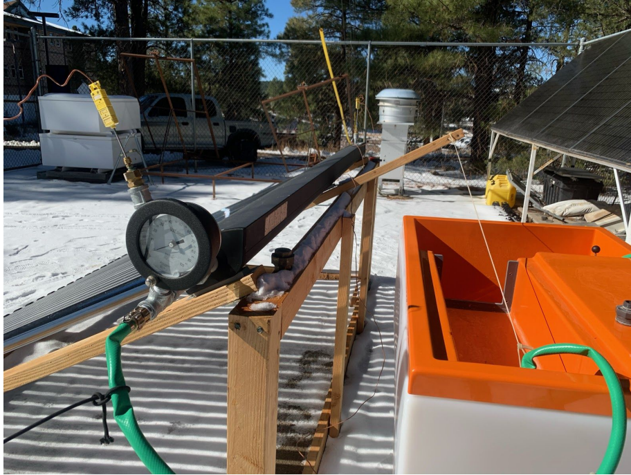
Figure 2. Configuration of hose connected to bench and panel
